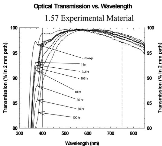
**FIGURE 6.** Phenyl Elastomer (1.57) Elastomer after Exposure to UV
