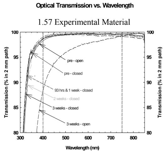
**FIGURE 7.** Phenyl Elastomer (1.57) after Exposure to Dry Heat (150°C)
