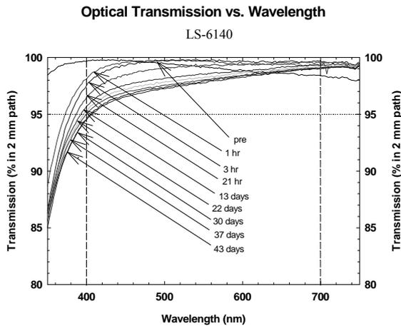
**FIGURE 5.** PDMS Elastomer after Exposure to UV
