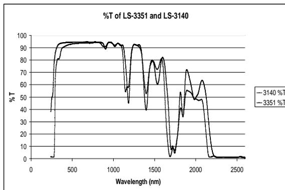
**FIGURE 3.** %Transmittance (%T) of 1.41, 1.51 Refractive Index gel. 1 cm thickness, quartz cuvette from 240 nm – 2600 nm
