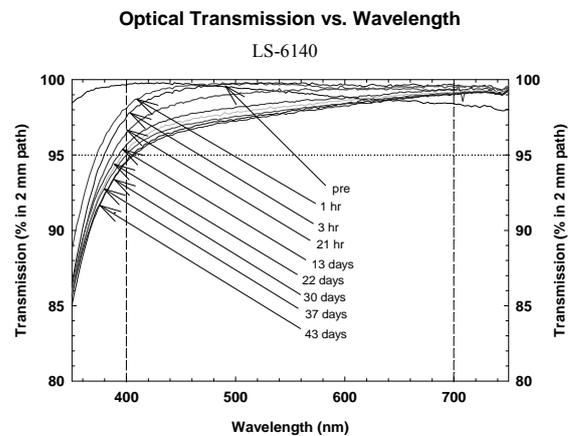
**FIGURE 4.** PDMS Elastomer after Exposure to Dry Heat (150°C)
