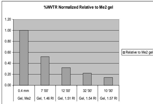
**FIGURE 2** Water Vapor Transmission Rate 40°C/90% RH/ 2mm Sample Thickness
