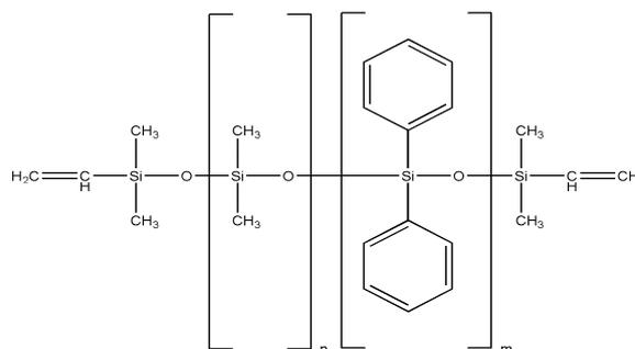
**FIGURE 1A.** Vinyl terminated polydiphenyldimethylsiloxane
